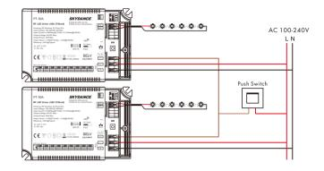
The provided AC Push-Dim interface allows for a simple dimming method using commercially available non-latching (momentary) wall switchs.
