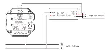
• Connect with 0/1-10V dimming driver (use AC OUT)
