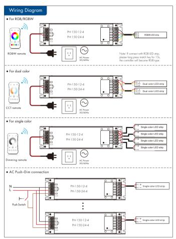
Note: Long press match key 5s, then short press match key 3 times, the light on/off time will be set to 3s, the indicator light blink 3 times. Long press match key 10s, restore factory default parameter, the light on/off time also restore to 0.5s.
