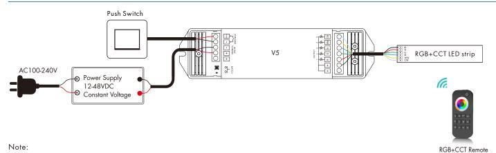
Long press match key 5s, then short press match key 3 times, the light on/off time will be set to 3s, the indicator light blink 3 times. Long press match key 10s, RGB and CCT light can not be on at the same time, the light on/off time restore to 0.5s (restore factory default). Long press match key 15s, RGB and CCT light can be on at the same time.
