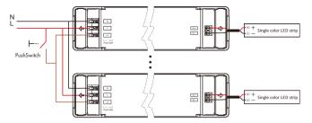
The provided AC Push-Dim interface allows for a simple dimming method using commercially available non-latching (momentary) wall switchs.
