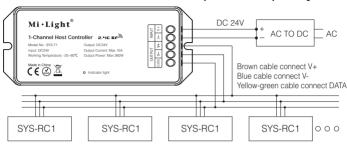
Note: When using "SYS-T1 controller", you need to add "SYS-T2 1-channel signal amplifier" for below 3 situations.
